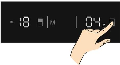
Press cooler set button until super cool symbol will be seen on the screen. Buzzer will sound beep beep. Mode will be set.
