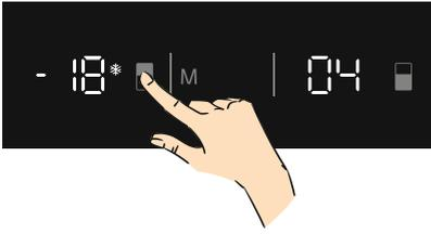
Press freezer set button until Super freeze symbol will be seen on the screen. Buzzer will sound beep beep. Mode will be set.
