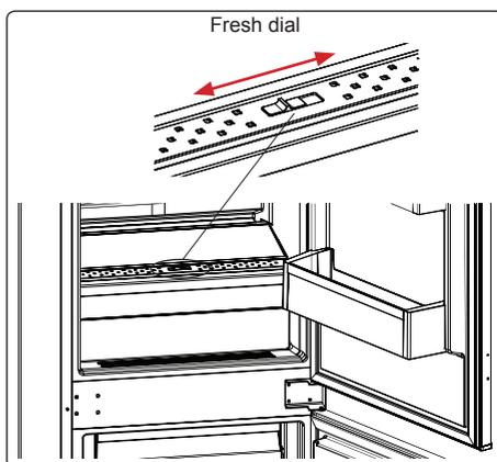
If the crisper is full, the fresh dial located in front of the crisper should be opened. This allows the air in the crisper and the
